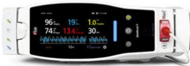
The Handheld snaps into the Docking Station to provide a fully featured standalone monitor. The Docking Station connects to AC power for standalone operation or charging of the Handheld. An optional Docking Station battery is available. The Standalone features Nurse Call, analog output, and serial output.
