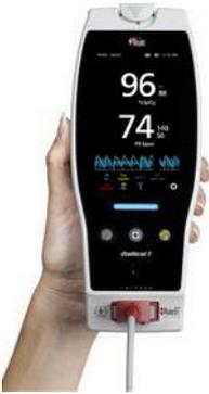
The Handheld contains the majority of the device features. All measurements and device status datum are displayed on the touchscreen. All user input is performed through the touchscreen and control buttons. The sensor cable connector is located on the Handheld.
